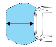
The RSS is automatically enabled when the gear selector is placed in R (Reverse) and the ignition is ON. The park aid disable switch allows the driver to disable the RSS only when the ignition is ON, and the gear selector is in R (Reverse). The OFF indicator remains illuminated when the system is disabled. If the
